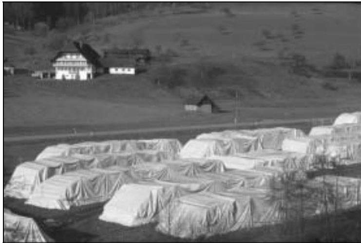
Photo 14: Log storage under O 2 exclusion in Germany (Source: FVA)
