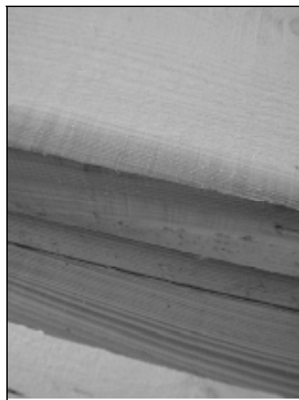
Photo 6: Peripheral discoloration of spruce (Source: CTBA)
